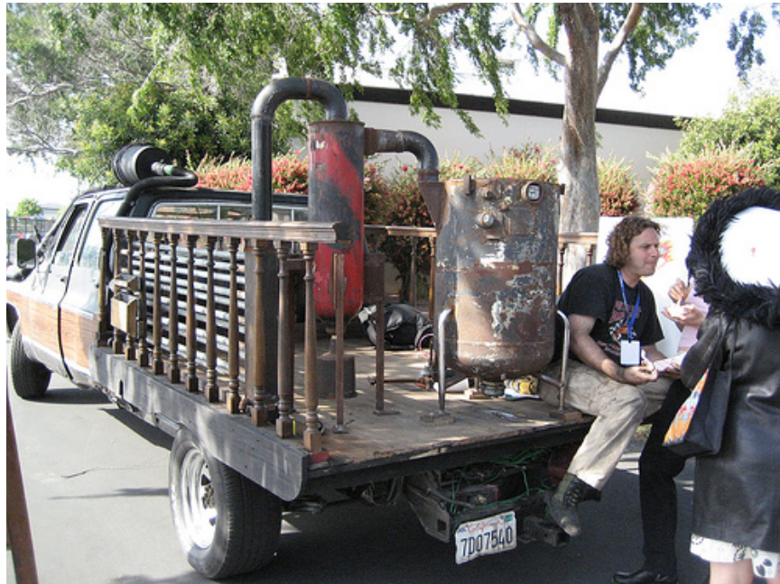
Figure 5: California Wood Burning Truck
